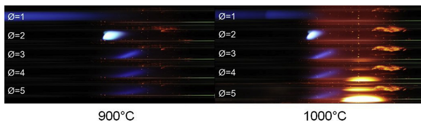
Fig. 3. Representative direct image of propane/air flame and soot responses with fixed 100 \text{ mL min}^{-1} total flow rate at 900^\circ\text{C} and 1000^\circ\text{C} and equivalence ratios from 1 to 5.
