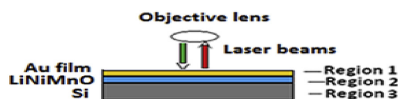
Fig. 1. Schematic illustration of geometry of laser incidence on the sample surface. For other samples, LiNiMnO is replaced by the other films. The two laser beams were focused to the same point although shown separate for clarity.
