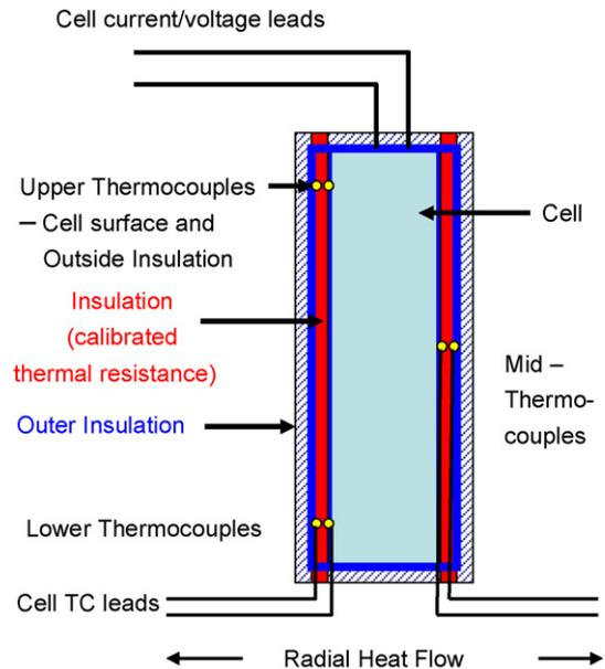
Fig. 8. Cell overcharge measurement fixture for determination of heat flow during overcharge and runaway.
