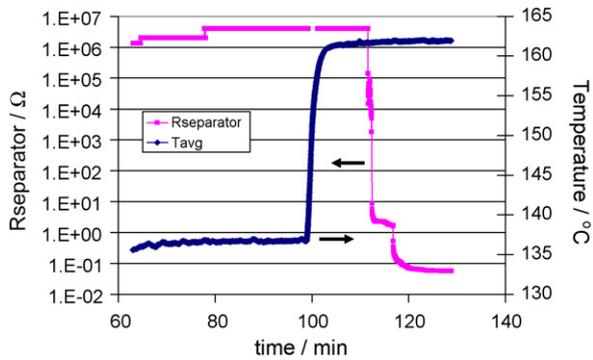
Fig. 6. Impedance of Celgard separator after ramp to temperatures above the PP melt temperature and the resulting short circuit failure of the separator after 8 min.
