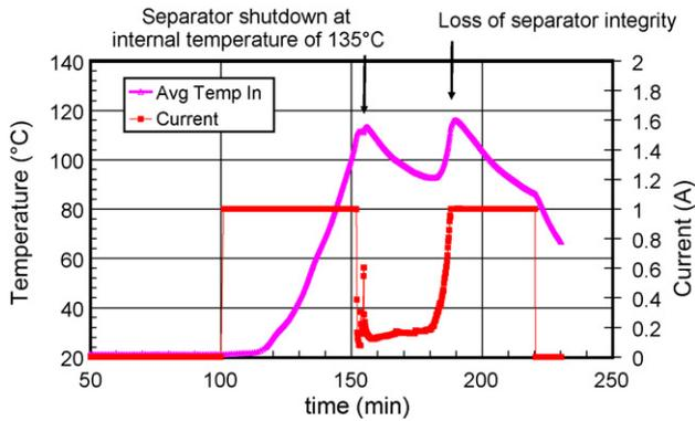
Fig. 10. Cell temperature and current profile during overcharge resulting in separator shutdown followed by delayed separator failure and runaway.
