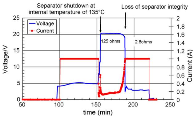
Fig. 11. Cell voltage and current profile during overcharge and subsequent runaway.
