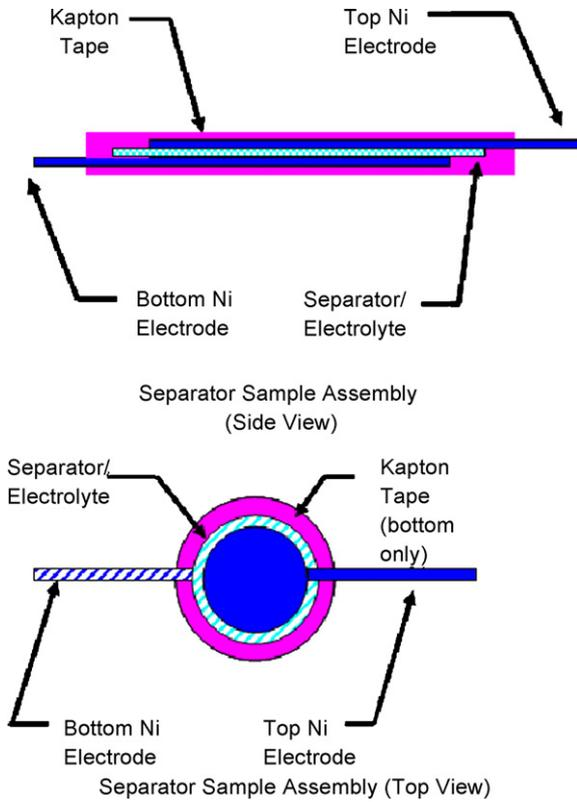
Fig. 1. Separator sample assembly for impedance measurements showing separator/electrolyte layered between Ni electrodes and sealed with Kapton tape.
