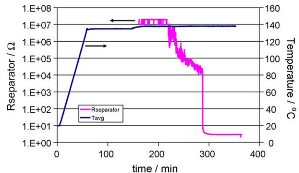
Fig. 5. Eventual breakdown preceded by slow degradation of cell dc resistance (>2 h).
