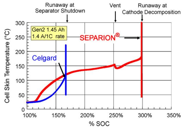
Fig. 13. Comparison of cell skin temperatures for cell with Celgard shutdown separator and cell with SEPARION® non-shutdown separator.
