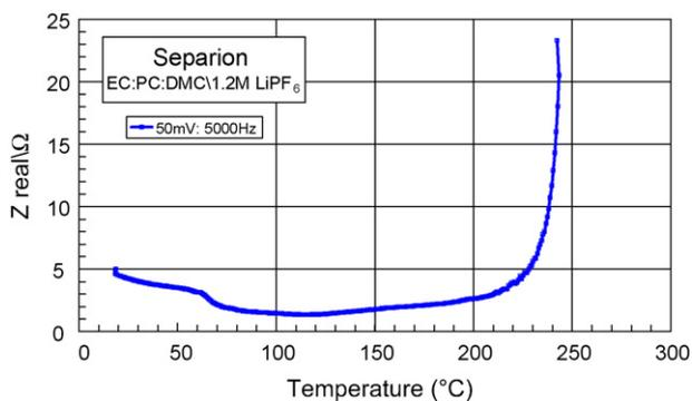
Fig. 7. Impedance profile of SEPARION® separator during a thermal ramp to 250 °C showing the non-shutdown, high-temperature stability of the separator.
