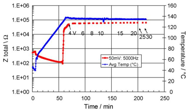
Fig. 4. No change in impedance after brief exposure to voltages up to 30 V.
