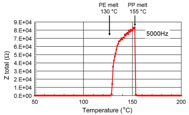
Fig. 3. Impedance (5 kHz) of Celgard Trilayer separator as a function of temperature (3° min<sup>-1</sup> ramp rate).
