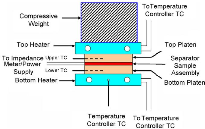
Fig. 2. Separator measurement fixture showing separator sample assembly between heated platens.
