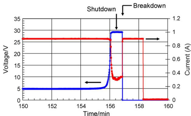
Fig. 12. Overcharge using higher power supply compliance voltage (30 V) resulting in more rapid separator failure and cell thermal runaway.
