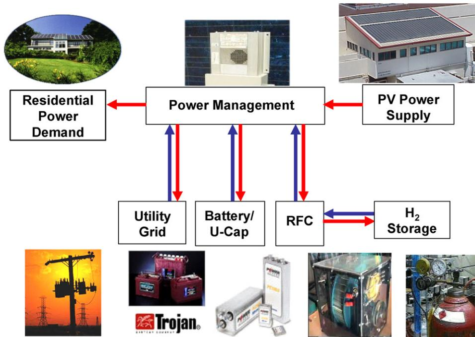
Fig. 1. Schematic of Simulink renewable RFC system model.
