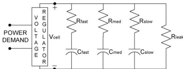
Fig. 2. R–C model of an ultra-capacitor system.
