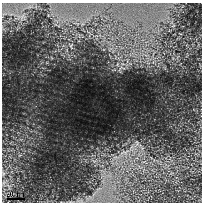
**Fig. 6.** TEM image of ordered mesoporous RuO<sub>x</sub>, the electro-oxidized product of ordered mesoporous Ru.
