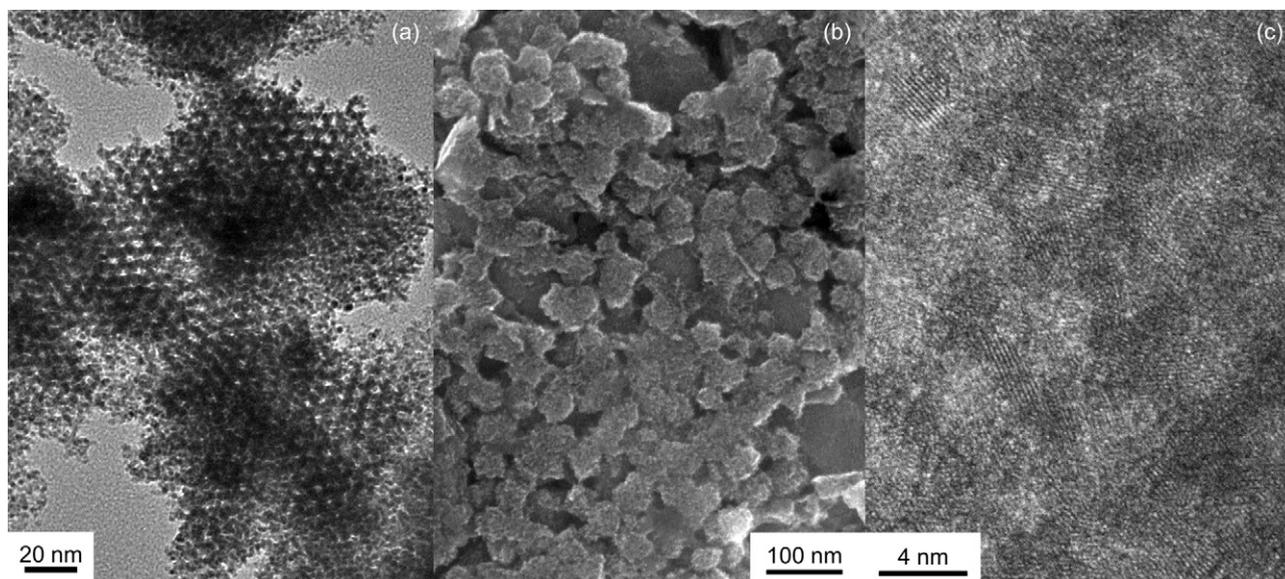
Fig. 2. (a, c) TEM and (b) SEM images of mesoporous Ru.
