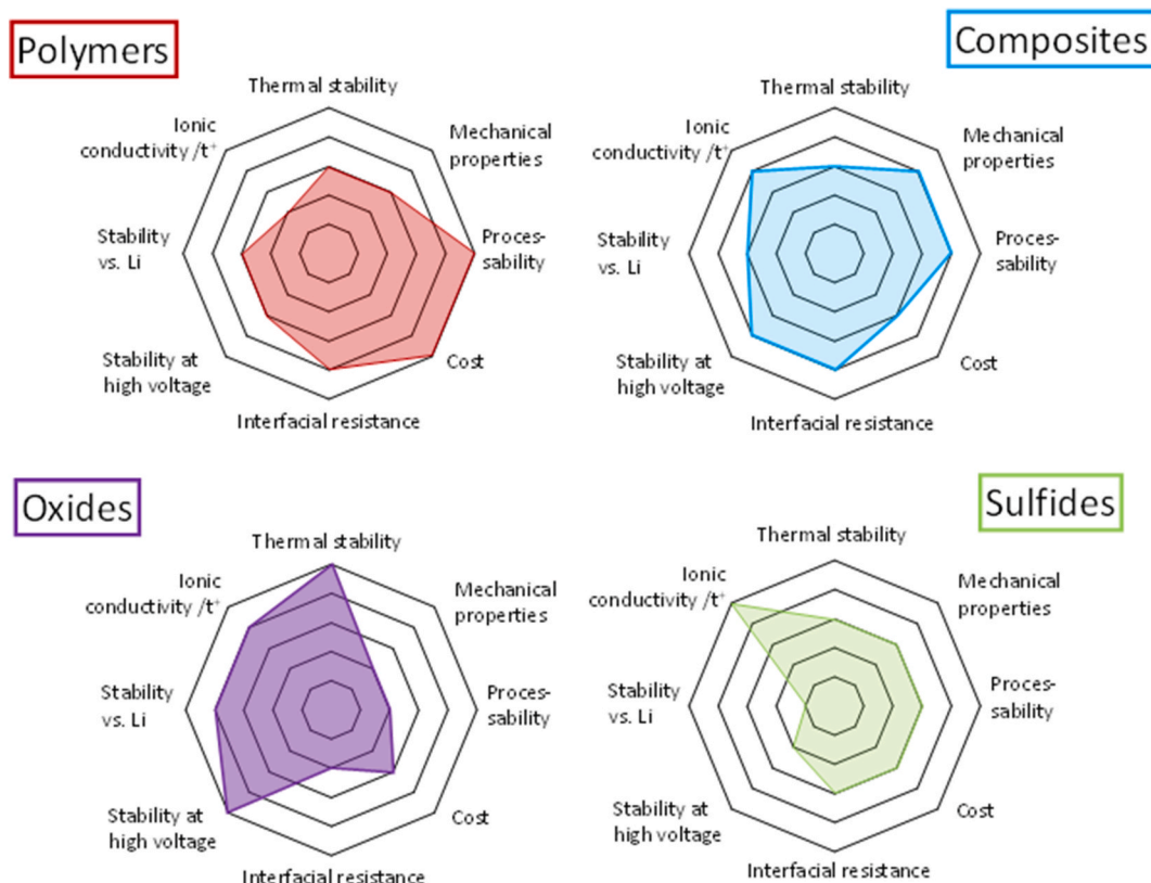
Fig. 7. Radar chart presenting the most relevant properties of the polymer, composite, oxide and sulfide families of solid-state electrolytes. The considered properties include chemical stability and electrochemical performance (Ionic conductivity and transference number ( t^+ ), stability against Li metal, stability against high voltage cathode, interfacial resistance), thermal and mechanical stability and cell integration towards manufacturing (described as processability and cost).
