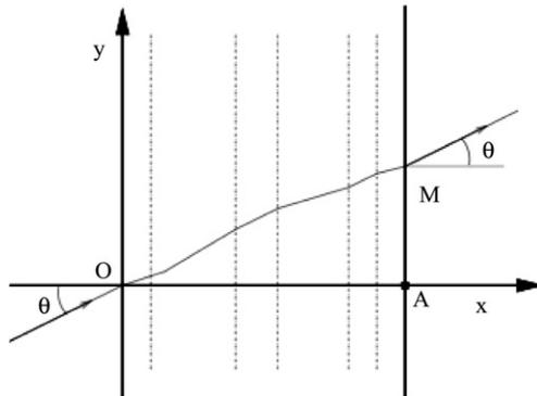
An incoming ray hits the system at the origin with an incident angle  $\theta$  and reappears after  $N$  refractions at  $M$  on the opposite side. Let  $\theta_k$  be the angle at which the luminous path meets the  $k$ th plate. The Snell–Descartes law states that  $n_k \sin \theta_k$  is independent of  $k$ . An easy computation shows that the length  $AM = \varphi(\theta)$  is given by
