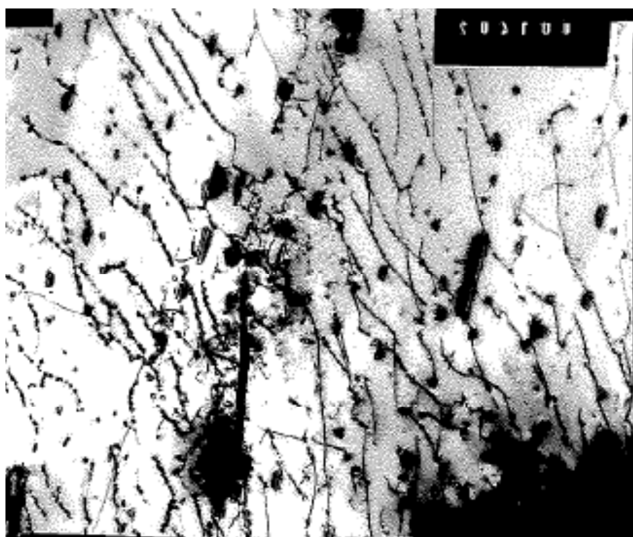
Figure 17: Thin-film transmission electron micrograph of Zircaloy-2 specimen showing dislocation lines decorated with hydride particles.
