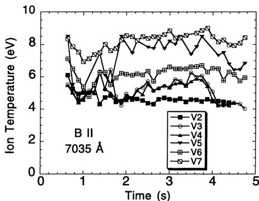
Fig. 3. Time histories of B II temperatures measured along the vertical views.
