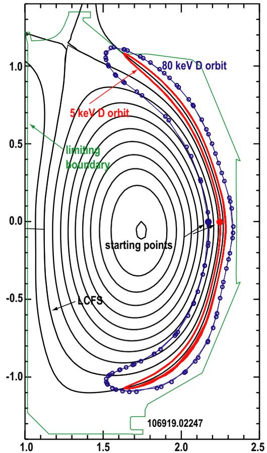
Fig. 4. Trapped ion orbits for 80 and 5 keV deuterium ions.
