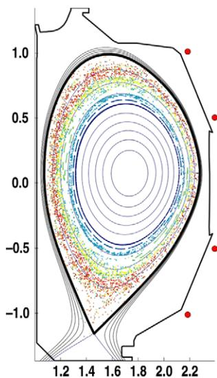
Fig. 1. Poincaré plot of 10 TRIP3D magnetic field line trajectories for 1000 toroidal transits for shot #122342 at 4650 ms with I-coil and C-coil. Also shown are the EFIT flux surfaces, EFIT separatrix, DIII-D inner vacuum vessel, and I-coil positions (red circles). (For interpretation of the references in colour in this figure legend, the reader is referred to the web version of this article.)
