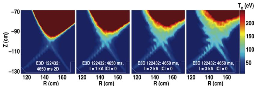
Fig. 4. 2D electron temperature distribution predicted by E3D on the  $\phi = 0$  plane for varying levels of even-parity I-coil current: 0, 1, 2, 3 kA. The separatrix tangle structure grows while the pedestal cools with increasing RMP strength.
