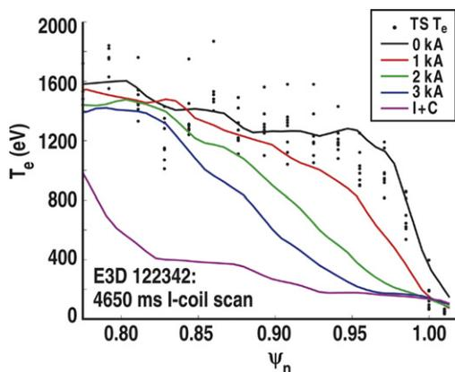
Fig. 5. The electron temperature pedestal sampled at the experimental Thomson scattering measurement location is predicted to cool as the I-coil current is scanned from 0 to 3 kA. The purple curve corresponds to the experimental settings: I-coil = 3 kA and C-coil = 12 kAt shown in Fig. 1.
