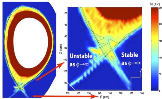
Fig. 2. The electron temperature contours computed by E3D closely follow the invariant manifolds that emanate from the X-point. The stable/unstable manifold oscillates wildly as it connects to the divertor target on the right/left hand side of the figure. The oscillatory behavior in  $T_e$  is an artifact of interpolation.
