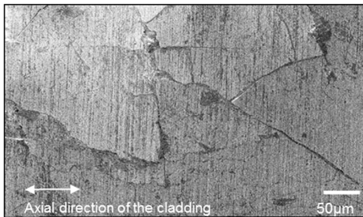
Fig. 9. SEM image of the cladding surface at the position ca.140 mm from the top end, after oxidation test in high air flow rate.
