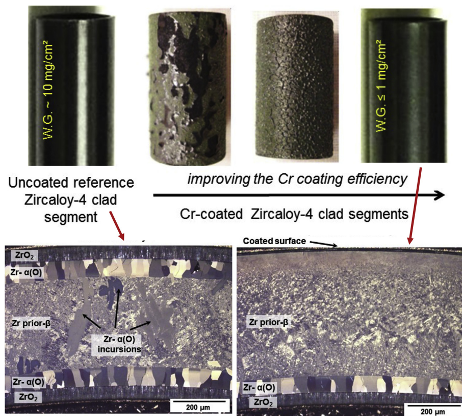
Fig. 11. Macrographs and optical (polarized light) of uncoated/Cr-coated Zircaloy-4 clad segments after steam oxidation for 300 s at 1200 °C followed by direct water quenching. Remark: because of the two-sided oxidation conditions applied, for the coated clad, the weight gain has been evaluated by subtraction of the contribution of the uncoated inner surface (calculated using the weight gain measured for the uncoated reference) 29.
