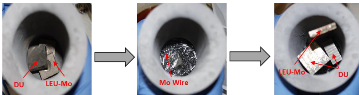
Fig. 1. Loading sequence, shown from left to right. A layer of smaller pieces of LEU-10Mo and DU are loaded first, the additional Mo is then added, and finally the larger LEU-10Mo and DU pieces.
