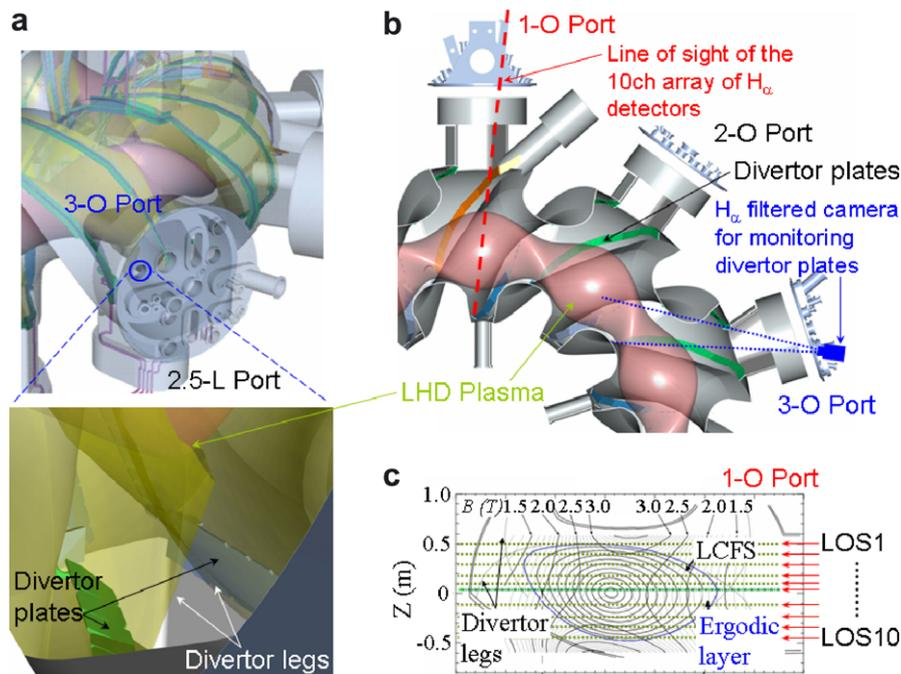
Fig. 1. (a) Bird's eye view of the LHD vacuum vessel with the pictorial view of the divertor region from the camera position, (b) cross-sectional view of the vacuum vessel with diagnostic systems for measuring neutral hydrogen in the plasma periphery, and (c) map of the magnetic surfaces and the magnetic field on the poloidal surface of the line of sight of a  $H_\alpha$  detector array.
