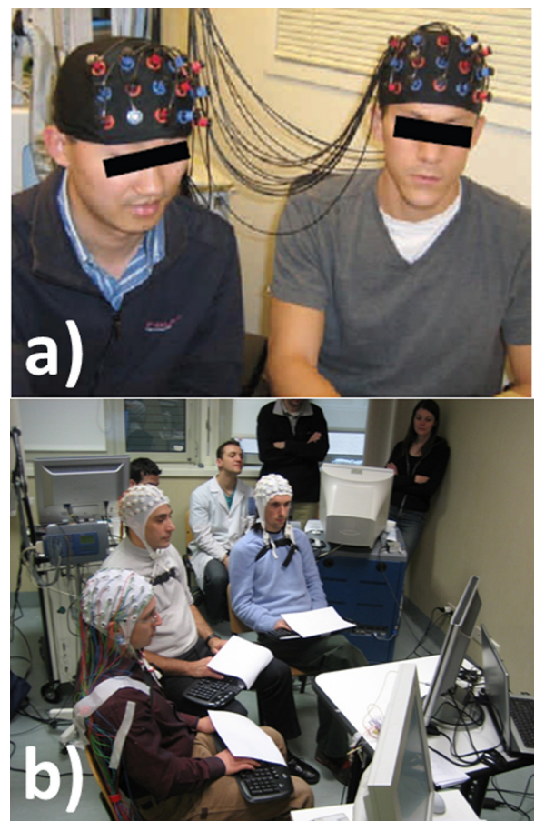
Fig. 5. Different hyperscanning devices for hemodynamic and electric modalities. The figure shows in the upper part (A) the split of the fibers to generate an NIRS hyperscanning device from one single NIRS device; in the lower part (B) the EEG hyperscanning setup during an iterated Prisoner's Dilemma task involving three subjects.
