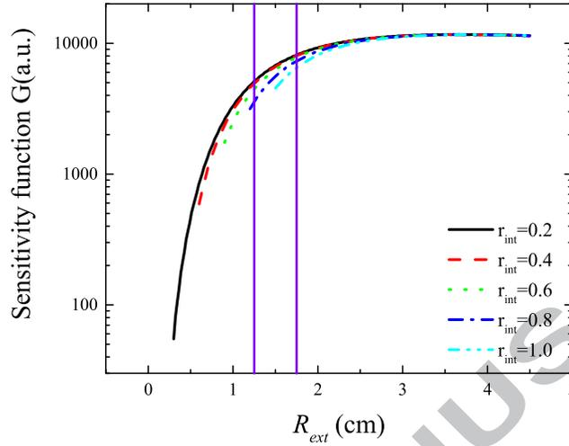
Figure 4: Sensitivity as a function of the the external radius for different values of the internal radius  $r_i$  of the pick-up coils.
