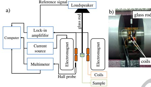
Figure 1: (a) Block diagram of the home-made VSM (b) Image of the vibrating sample magnetometer indicating the pick-up coils placement and the glass rod that supports the magnetic sample.
