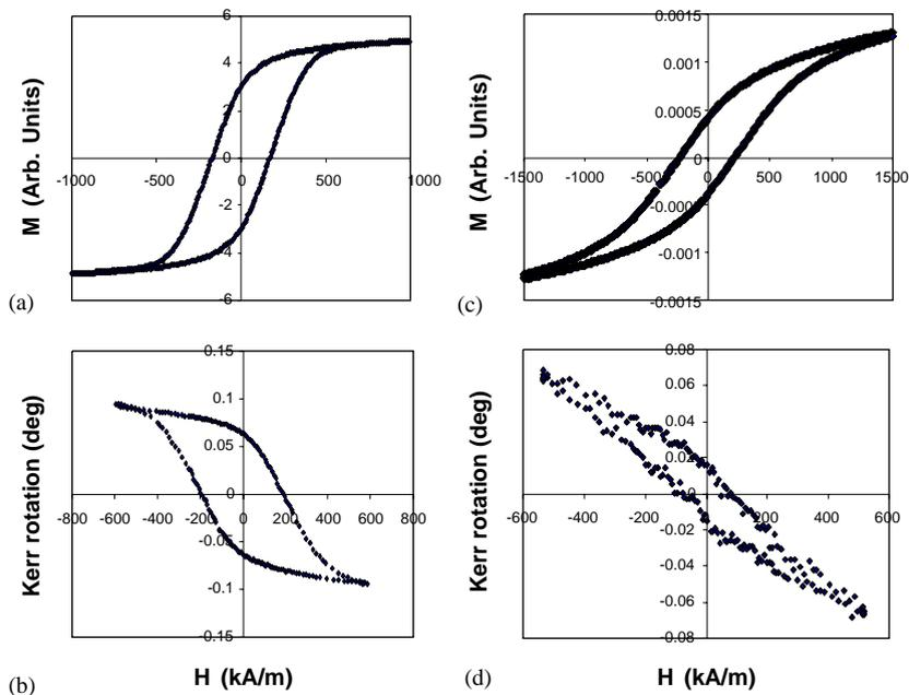
Fig. 4. (a) Magnetic and (b) Kerr loops of  $\text{BaFe}_{12}\text{O}_{19}$  film (200 nm thick). (c) Magnetic and (d) Kerr loops of  $\text{CoFe}_2\text{O}_4$  film (180 nm thick). Note the difference in the respective scales of the loops.
