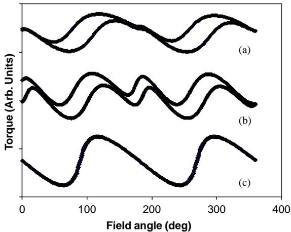
Fig. 3. Torque curves of (a) thin (60 nm), (b) thick (180 nm)  $\text{CoFe}_2\text{O}_4$  films and (c) 200 nm thick  $\text{BaFe}_{12}\text{O}_{19}$ .
