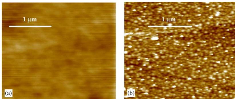
Fig. 1. (3  $\mu\text{m} \times 3 \mu\text{m}$ ) AFM images of (a) CoFe<sub>2</sub>O<sub>4</sub> and (b) BaFe<sub>12</sub>O<sub>19</sub> thin films epitaxially grown on (100) MgO and (001) Al<sub>2</sub>O<sub>3</sub>, respectively.
