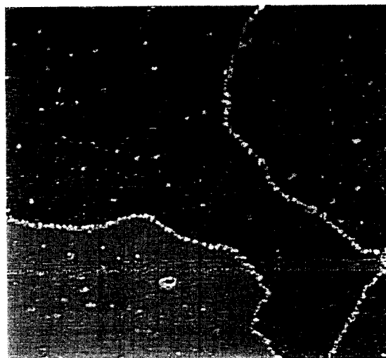
Fig. 6. Image of the Al(111) surface after deposition of a small amount of \text{H}_2\text{S} . Bright features at the step and on the terraces are due to S clusters. 700 \text{ Å} \times 640 \text{ Å} , I = 1 \text{ nA} , V = -1.5 \text{ V} , T_{\text{ads}} = 570 \text{ K} , 12 \text{ L H}_2\text{S} .
