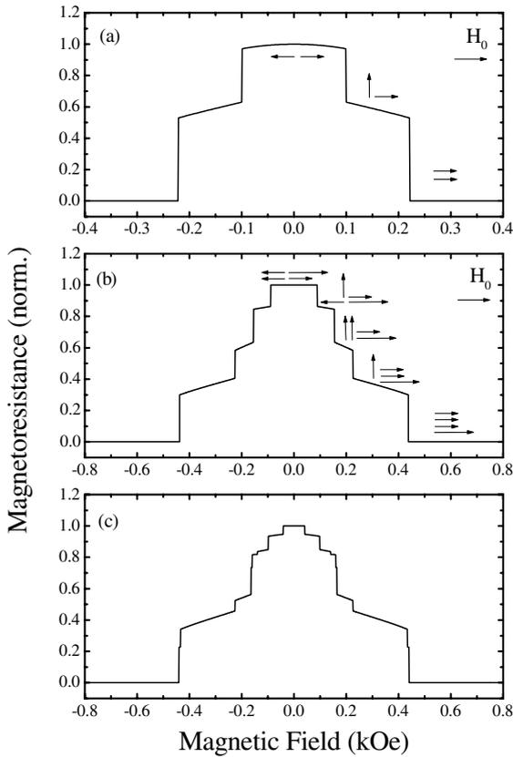
Fig. 1. Magnetoresistance versus applied field  $H_0$  for the (a)  $N = 3$ , (b)  $N = 5$  and (c)  $N = 7$  Fibonacci generations. The parameters are  $r \sim 0.33$  and a cubic anisotropy field  $H_{ca} = 0.5$  kOe.
