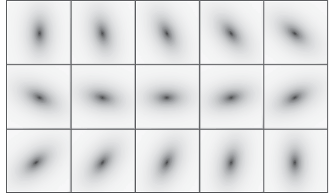
Fig. 4. Example of SEs obtained with a variation of orientations convolved with a Gaussian point spread function.
