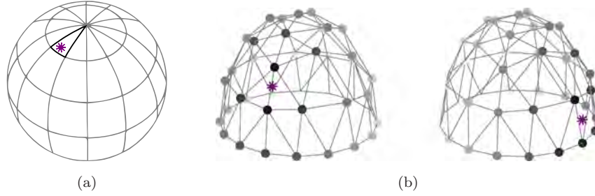
Figure 5: Bin distributions resulting from (a) angular thresholds in spherical angles (bins represented as areas) and (b) the adopted tessellation-based approach (bin centers represented as dots). Our 3D descriptor uses a parametrized division of the sphere to create the voting bins that avoids the typical meridian division that over-represents the zone near the north pole. Examples of vote patterns are shown, where the purple asterisk indicates the coordinates of the normal vector.
