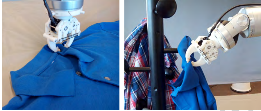
Figure 10: Detail of the gripper and the hanging operation.
