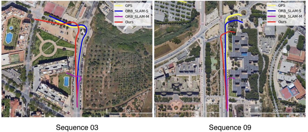
Fig. 13. Qualitative tests on Malaga dataset exhibited on Google Earth. The blue and purple trajectories express stereo and monocular ORB-SLAM respectively, with the yellow one represents GPS(ground truth). Our performance(PoseConvGRU-cons) shows in red (best viewed with zoom-in).
