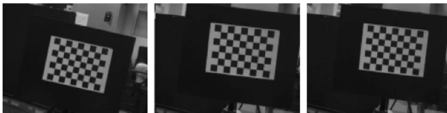
Fig. 4. Three images of the chessboard used to calibrate with Zhang's algorithm, taken with different position and attitude. The sequence was taken by a Sony DSC-S50 digital camera (target size of 640 \times 480 pixels) with its minimum focal length ( f = 6.1 mm).
