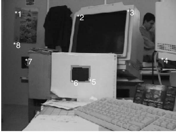
Fig. 6. The square is taken as target in the initial image. The deformation of the contour fitted to it allows us to recover the heading direction and epipolar lines. The latter will be computed for the indicated points, as an example.
