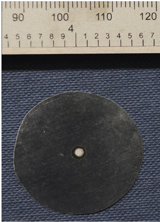
Fig. 3. Molybdenum target for X-ray generation showing the beam spot.
