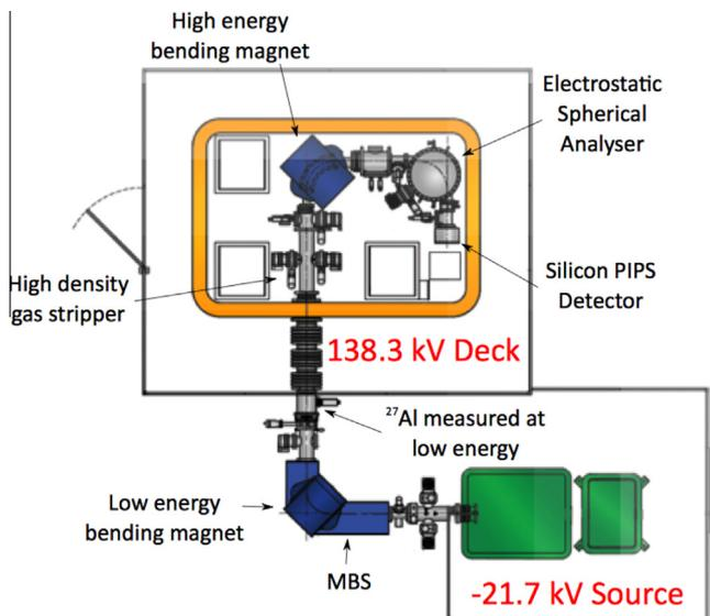
Fig. 1. Schematic of the SSAMS used for <sup>26</sup>Al-AMS (courtesy of NEC).
