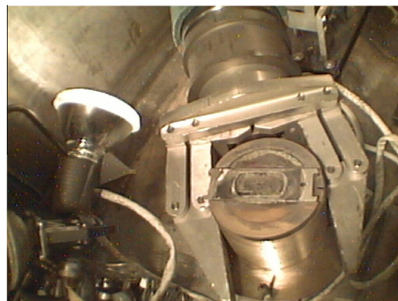
Fig. 3. View of the ^{252}\text{Cf} deposit held by a manipulator in the hot cell facilities at the HFIR reactor. The source is visible as a roughly 5 cm by 2 cm deposit in the center of the support plate. All operations on the source must be done remotely and as a result no cleaning of the plate and deposit for UHV operation is possible.
