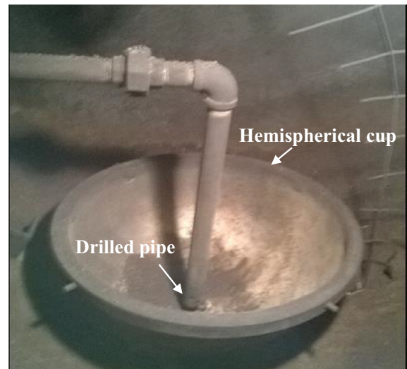
Fig. 3. Calibrated drilled pipe hemispherical disperser.
