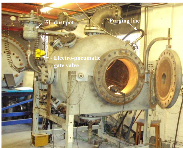
Fig. 2. Modified 1 \text{ m}^3 dust explosion vessel.
