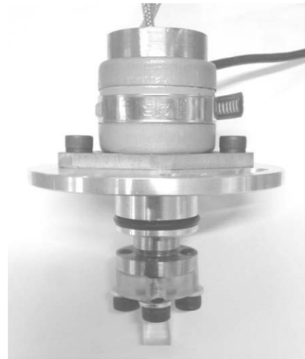
Fig. 7. Optical nozzle full assembly.
