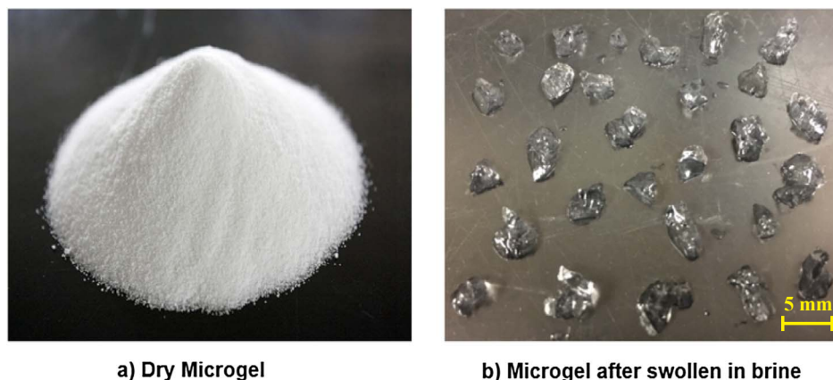
Fig. 2. Microgel before and after being swollen in sea water.
