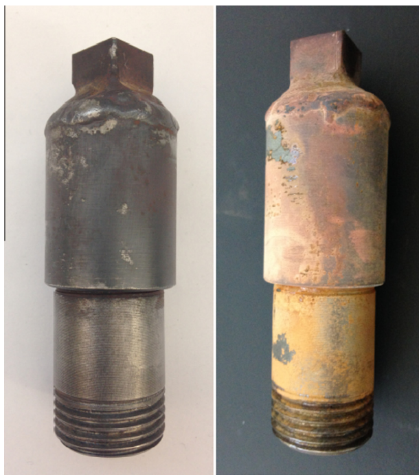
Fig. 4. Fouling on deposition probe after test O1 (right side).
