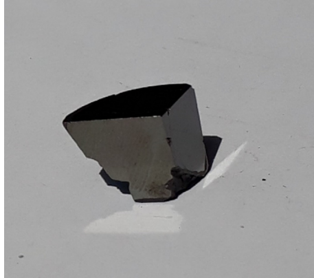
Fig. 2. Coal core sample polished and carbon-coated for SEM analysis.
