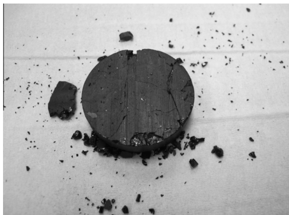
Fig. 14. The photograph of the Cottage Grove bituminous coal (CGC-S2) core after it underwent shockwave experiments.
