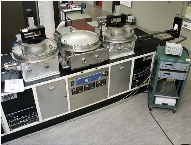
Fig. 1. The pilot system (PILOT) used for demonstrating HWCVD on moving substrates.
