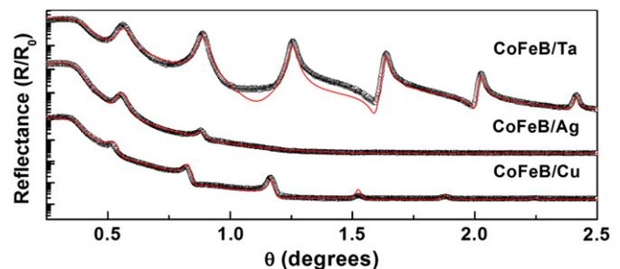
Fig. 2. XRR experimental patterns (black empty circles) for our multilayer films, together with the experimental data fittings/simulations (red solid lines). The main parameters obtained through the XRR experimental data fitting for each multilayer thin film are presented in Table 1.
