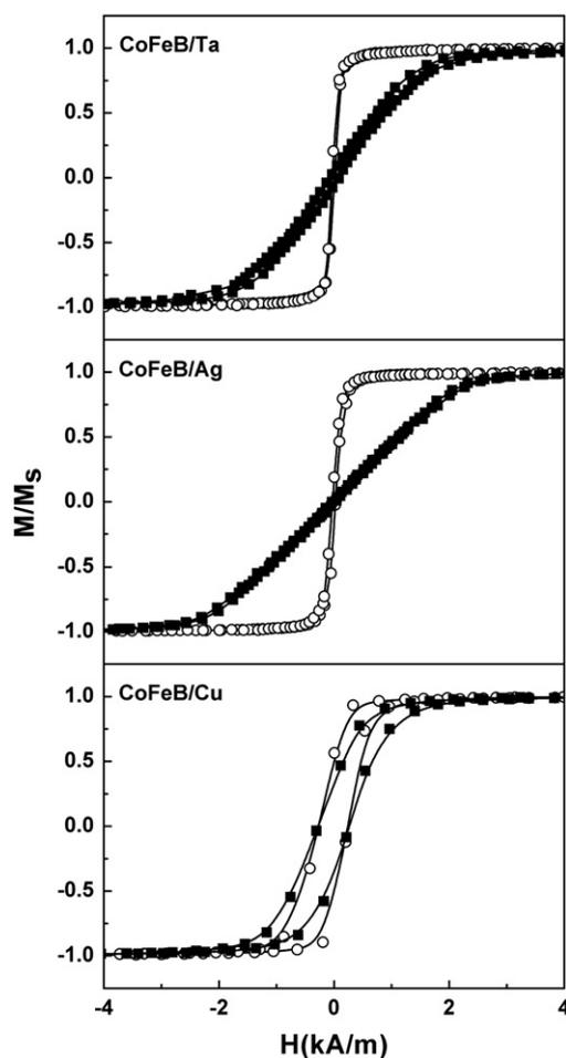
**Fig. 3.** Magnetization curves for the CoFeB/Ta, CoFeB/Ag and CoFeB/Cu samples, obtained when the magnetic field is applied along (open circles) and transversely (closed squares) to the direction defined by the magnetic field applied during the deposition, i. e., perpendicularly to the main axis of the sample.
