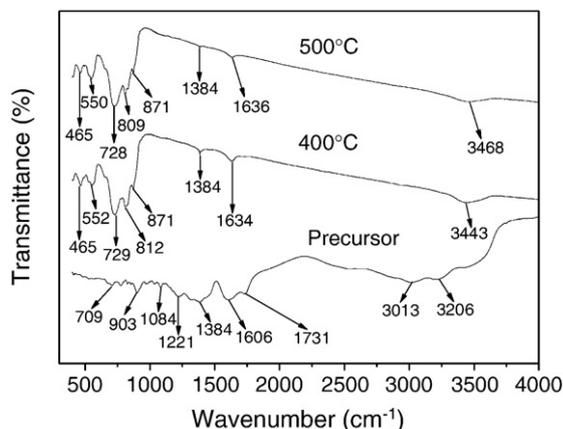
Fig. 5. FT-IR spectra of precursor samples recorded at various temperatures in air.
