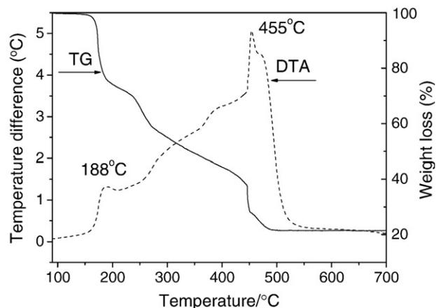
Fig. 4. TG-DTA analysis of the precursor samples.
