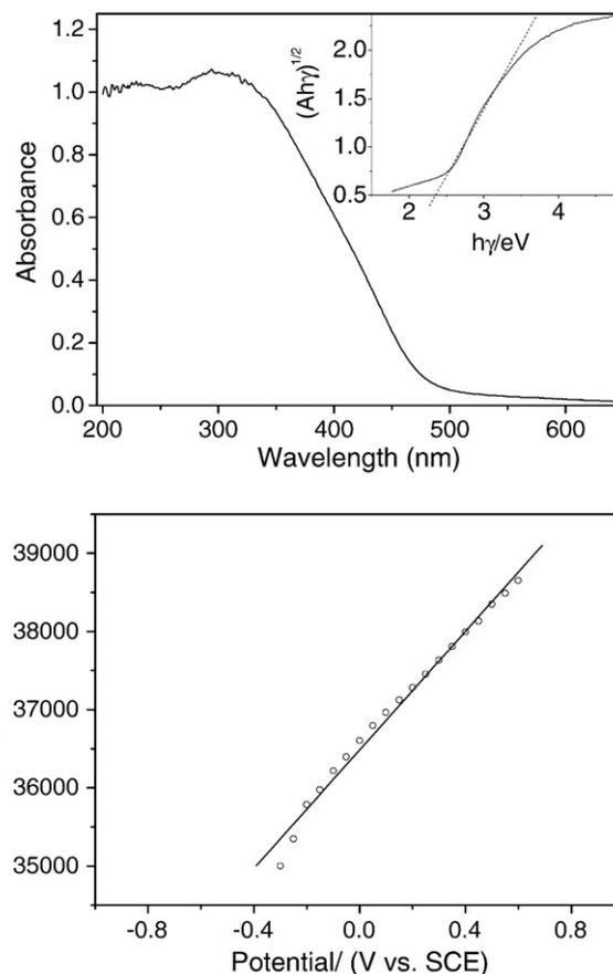
Fig. 9. UV–Vis diffuse reflectance spectroscopy of the  $\gamma$ - $\text{Bi}_2\text{MoO}_6$  powder and Mott–Schottky plot of the  $\gamma$ - $\text{Bi}_2\text{MoO}_6$  film in 0.1 M KCl solution (the frequency of the ac signal was 1 kHz).
