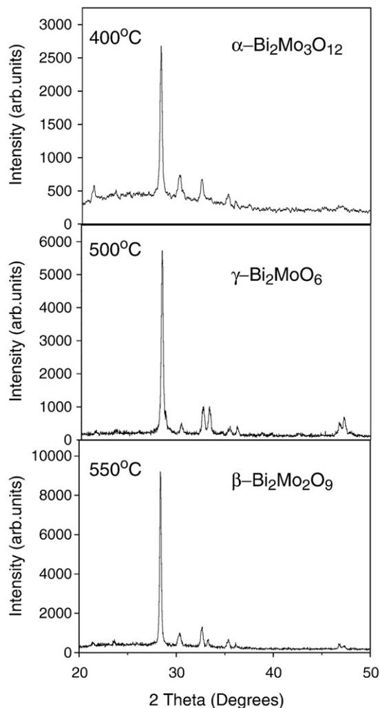
Fig. 2. X-ray diffraction analysis of the precursor film treated at various temperatures for 1 h.
