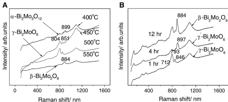
Fig. 1. Raman spectroscopy of the precursor film treated at various conditions. A, different temperatures for 1 h; B, different time at 500 °C.
