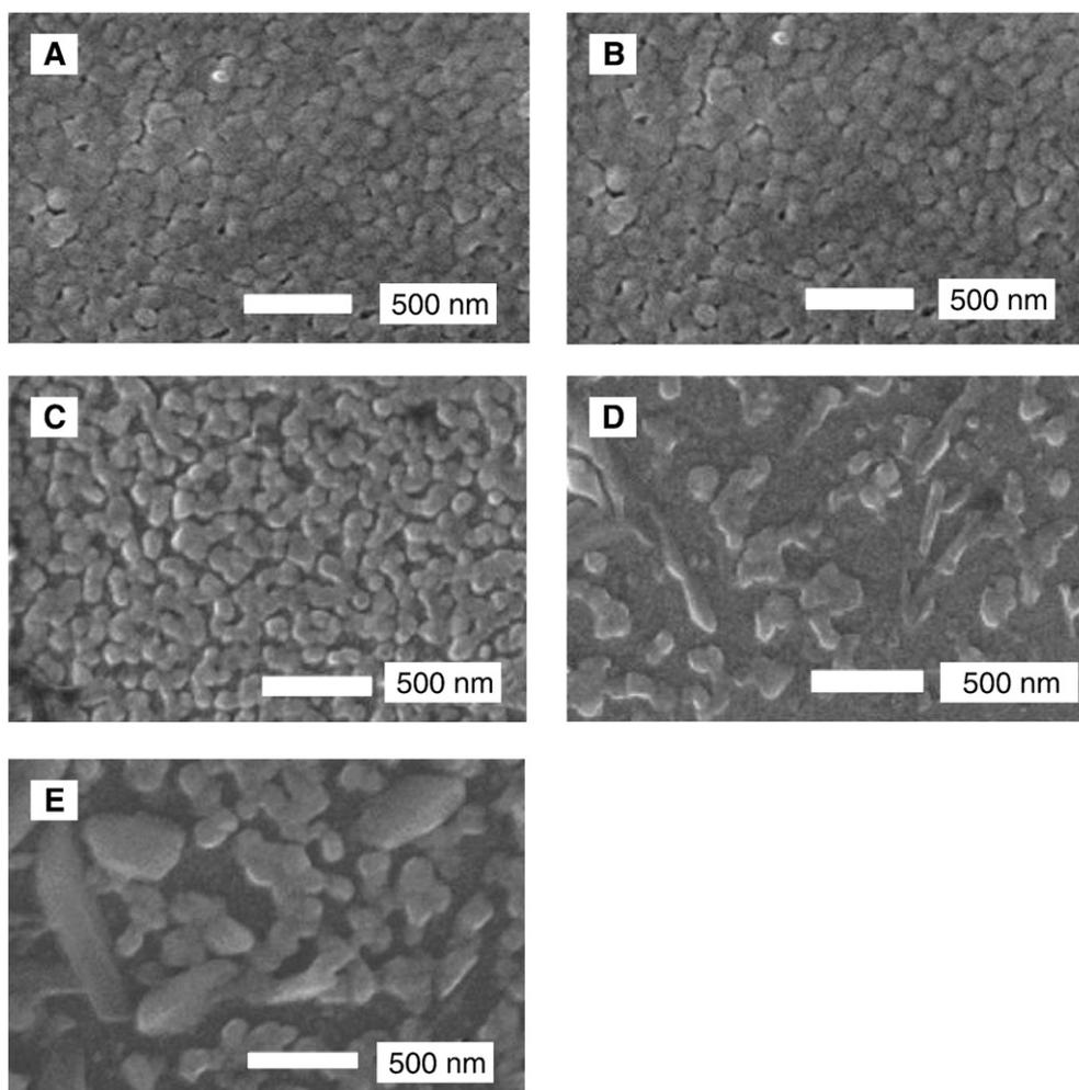
Fig. 3. SEM of the precursor film treated at various conditions (A, Precursor; B, 400 °C for 1 h; C, 500 °C for 1 h; D, 500 °C for 4 h; E, 500 °C for 12 h).
