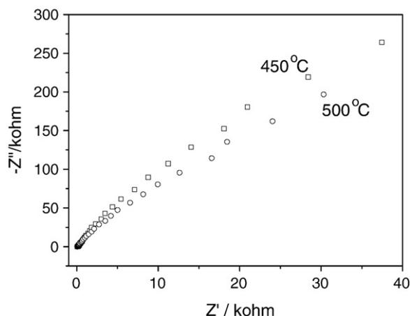
Fig. 7. Electrochemical impedance spectra plane display of the  $\gamma$ - $\text{Bi}_2\text{MoO}_6$  film samples treated at 450 °C and 500 °C.
