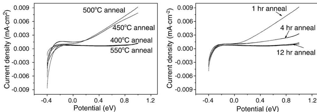
Fig. 6. Photocurrent response for the film samples treated at various conditions versus the applied bias potentials under visible light irradiation ( $\lambda > 420 \text{ nm}$ ) with light intensity of 150  $\text{mW}/\text{cm}^2$ . A, different temperatures for 1 h; B, different time at 500 °C.
