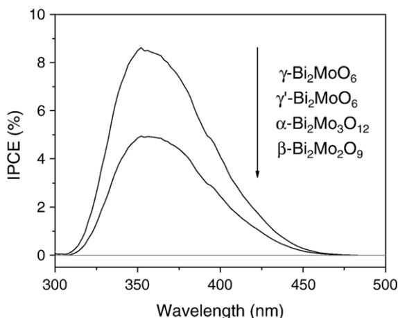
Fig. 8. IPCE vs.  $\lambda$  for the  $\alpha$ - $\text{Bi}_2\text{Mo}_3\text{O}_{12}$ ,  $\beta$ - $\text{Bi}_2\text{Mo}_2\text{O}_9$ ,  $\gamma$ - $\text{Bi}_2\text{MoO}_6$ , and  $\gamma'$ - $\text{Bi}_2\text{MoO}_6$  film electrode in 0.1 M KCl solution at various potentials under monochromatic light irradiation.
