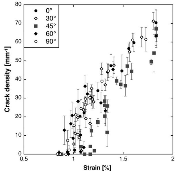
Fig. 5. Crack density vs. strain for S2S processed ITOA coatings on PET at different in-plane loading orientations.
