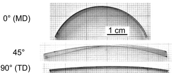
**Fig. 9.** Photographs of S2S processed ITOA/PET film samples along MD ( $\theta=0^\circ$ ) and TD ( $\theta=90^\circ$ ), and at a 45° orientation.
