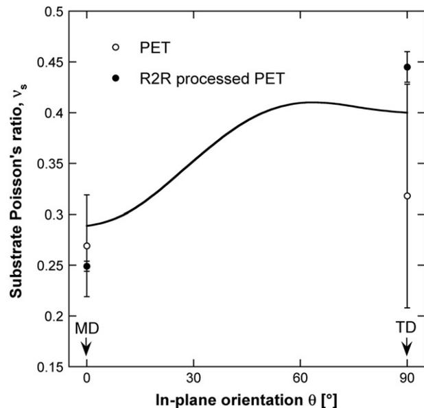
Fig. 3. Effective Poisson's ratio of the PET substrate as a function of in-plane orientation. The curve represents Eq. (3).
