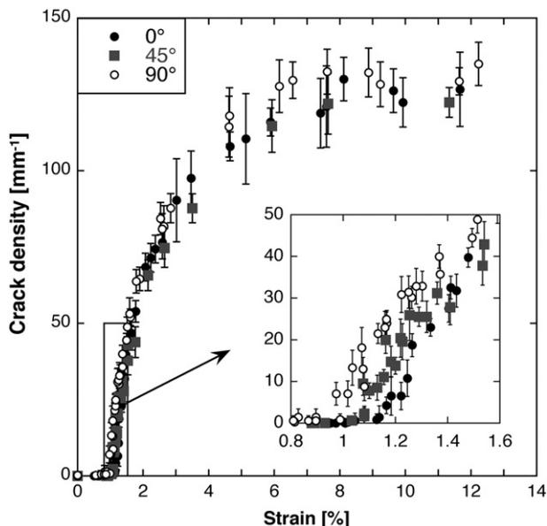
Fig. 7. Crack density vs. strain for R2R processed ITOA coatings on PET at different in-plane loading orientations.
