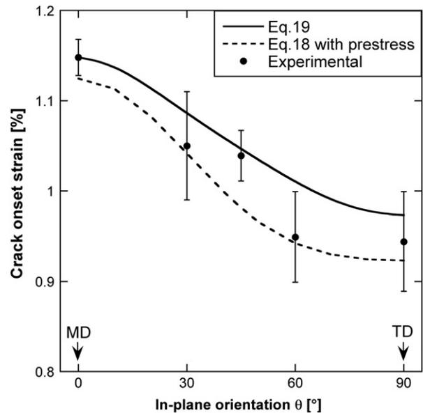
Fig. 8. COS variation with in-plane loading angle  $\theta$  for R2R films with a 4 N preload during fragmentation testing. Eq. 18 including pre-stress (isotropic substrate and same Poisson's ratio for coating and substrate) and Eq. 19 (anisotropic substrate and different Poisson's ratio for coating and substrate) are compared with experimental data.
