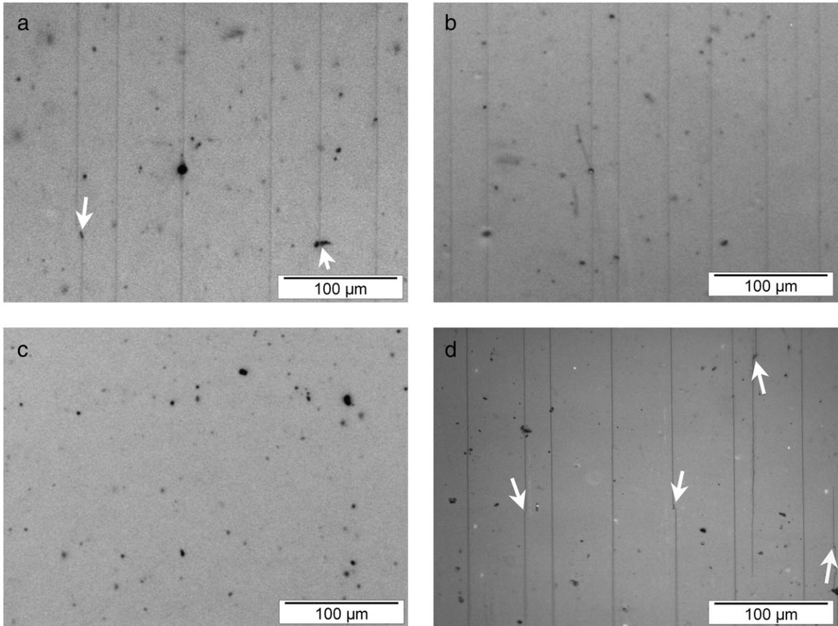
Fig. 4. Influence of process and substrate anisotropy on the damage state in the ITOA coating on PET under 1.1% strain (a: S2S film loaded along MD; b: S2S film loaded along TD; c: R2R film loaded along MD; and d: R2R film loaded along TD). The loading direction was parallel to the scale bar in the micrographs. Cracks are evident in all cases except for the R2R film loaded along MD. The arrows indicate defect initiation sites.
