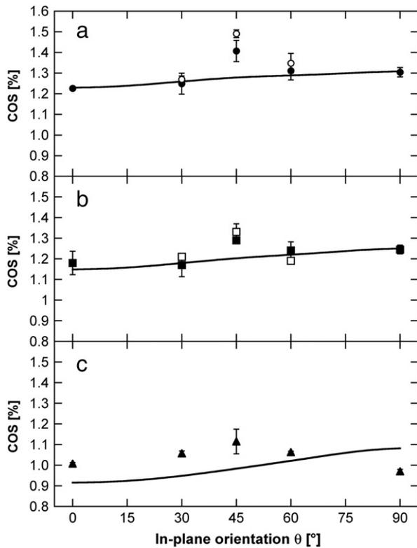
Fig. 6. COS variation with in-plane loading angle  $\theta$  for S2S films with no preload (a) and with 1 N (b) and 4 N (c) preloads during fragmentation testing. Black and open symbols are for positive and negative  $\theta$  values, respectively. The curves represent Eq. (19), with factors  $A$  and  $B$  given by Eq. (13).
