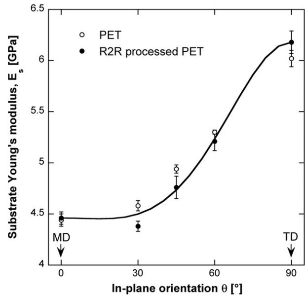
Fig. 2. Young's modulus of the PET substrate as a function of in-plane orientation. The curve represents Eq. (2).
