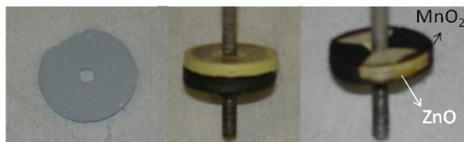
Fig. 1. Three different target configurations used for PLD deposition of thin films, bilayers and thin multilayers. Left, ceramic mixture of ZnO and MnO 2 , center: ZnO (top) and MnO 2 (bottom) targets for thick multilayer growth, right “cake” pellet of ZnO and MnO 2 for thin multilayer growth.
