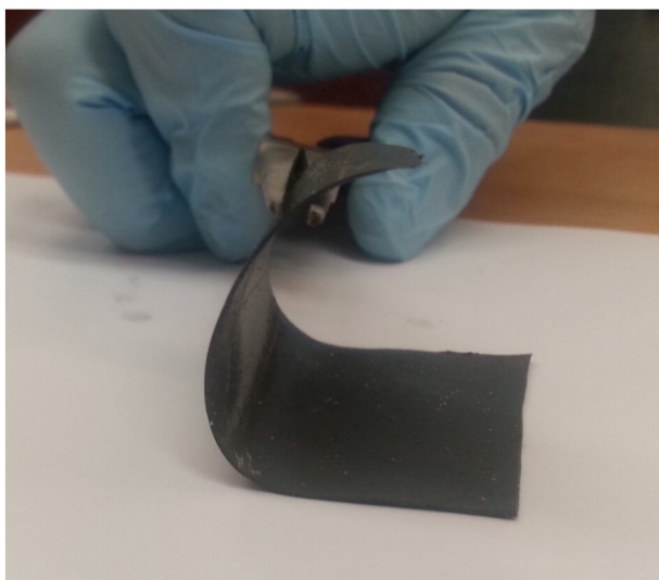
Fig. 2. Photograph of flexible free standing energetic film being rolled onto itself.
