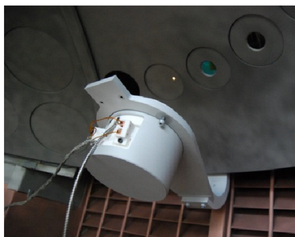
Fig. 2. Optical broadband monitoring system OptiMon™, illumination device mounted in the deposition chamber (left) and graphical user interface (right).
