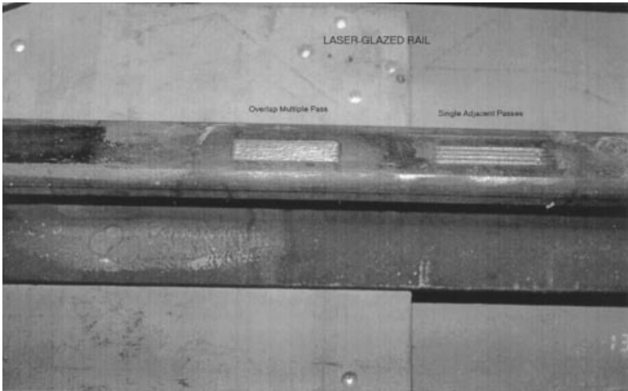
Fig. 14. A photograph of a section of unused railroad rail that received two 10 cm (4 in) long laser glaze treatments on its top surface: a multiple overlapping pass treatment done with a circular beam (left), and a multiple pass treatment made up of single adjacent passes done with an elliptical beam (right).
