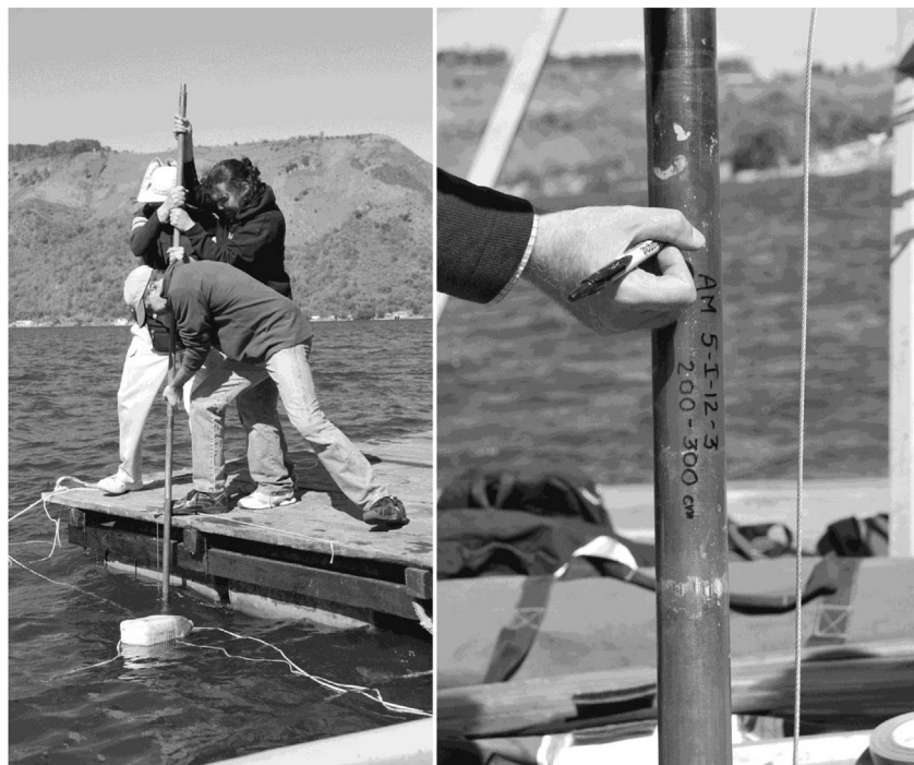
Fig. 5. Coring Lake Amatitlán using modified Livingston piston corer with locking piston, and labeling one of the core tubes representing a 1 m drive (200–300 cm core depth).
