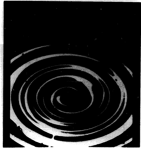
Fig. 2. Surface deformation at the vertical of a jet, for increasing values of the adimensional parameter \varepsilon = (F - F_c)/F_c . ( \phi = 1.44 mm; h = 10 mm): (a) \varepsilon = -0.2 ; (b) \varepsilon = -0.1 ; (c) \varepsilon = 0 : a transition is observed where the bump starts oscillating at a high eigenfrequency; (d) surface waves generated by the oscillatory motion of the bump. In both panels (c) and (d), stroboscopic lighting is used to visualize the phenomenon. In panels (a)–(c), the zoom magnification factor is 20.
