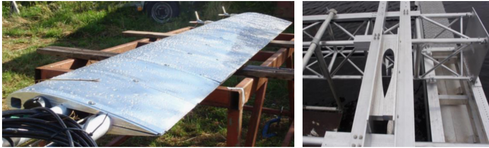
Fig. 7. Assembled hydrofoil strut (left) and hydrofoil clamp in place on the towing rig (right).
