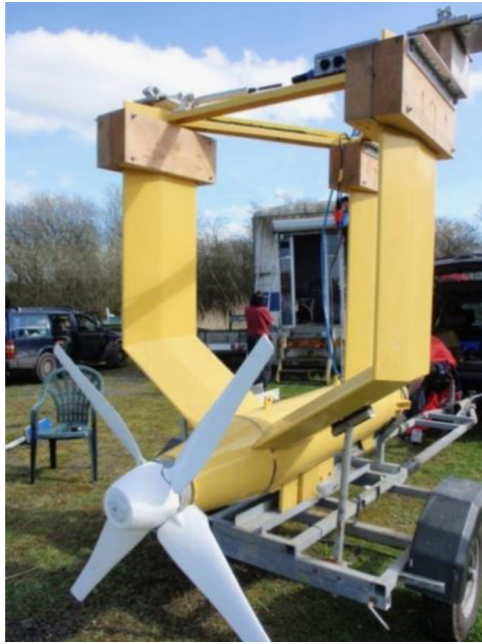
Fig. 3. Evopod 1:10th scale test model.
