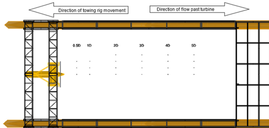
Fig. 4. Plan view of Evopod positioned on the towing rig and the ADV measurement matrix downstream.
