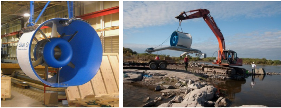
Fig. 1. Clean Current's diffuser, oblong in cross section at the exit, combines the benefits of maximizing the blade diameter for peak performance with containment of the rotating blades to prevent accidental impact on marine life (left), and the turbine being deployed in the Winnipeg River to field test in a remote community application using local equipment (right). (Photos courtesy of Clean Current).
