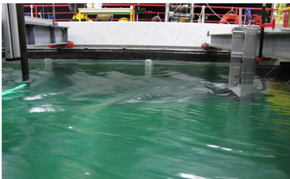
Fig. 5. MRL turbine mounted in the Wave-Current Circulation tank.
