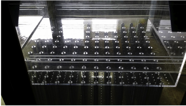
Fig. 6. Illustration of long platform supported by piles for 2D problem.
