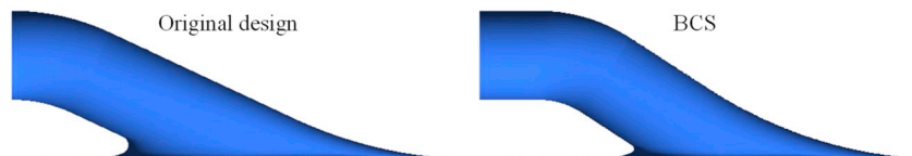
Fig. 7. Comparison between the original intake duct and the best compromise solution (BCS).
