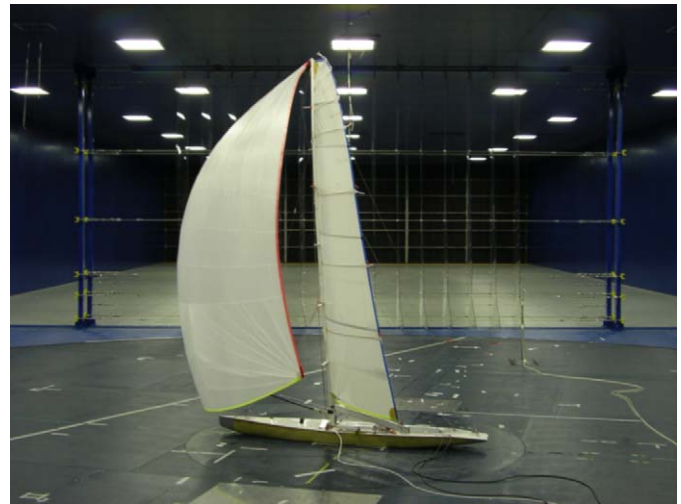
Fig. 2. Lunarossa model scale in the boundary layer test section of the Politecnico di Milano twisted flow wind tunnel sailing at 45^\circ AWA.
